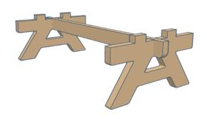
Step 2: Beam should fit flat between tabs.
