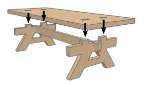
**Step 3:** Slide the table top down onto four tabs.
