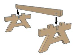
**Step 1:** Slide the beam down onto both legs.
